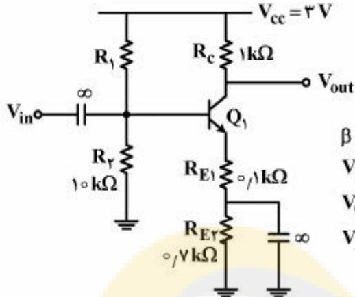
$$\begin{aligned}\beta &\gg 1 \\ V_{BE, on} &= 0.7 \text{ V} \\ V_{CE, sat} &= 0.7 \text{ V} \\ V_A &= \infty\end{aligned}$$
